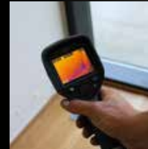
Find air infiltration problems
